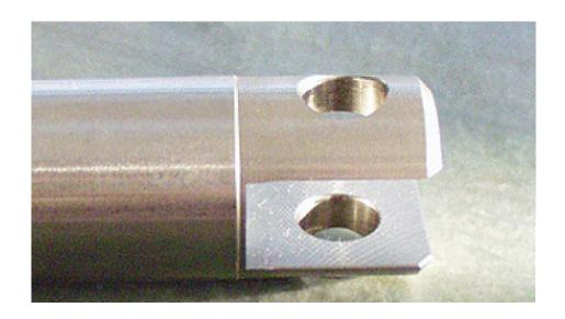
A steel clevice deburred by the COFA deburring tool. The manufacturer is running the tool at 1200rpm and 0.25mm/rev. Blade life is approximately 3,000-4,000 holes.
