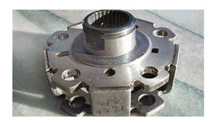
Another automotive component supplier manufactures steel reactionary gear carriers on a rotary transfer machine. They use DEFA tool to get precise chamfers inspite of the very large burrs caused by the drilling process.
