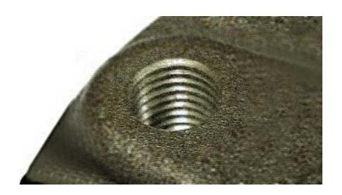
The unique design of the DEFA chamfering blades allows for chamfering threaded holes after tapping and without any damage to the threads. In this low carbon steel flange the DEFA tool runs at 1200rpm and 0.03mm/rev.
