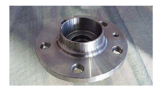
Drilling and chamfering in one operation saves cycle time and tool space.
