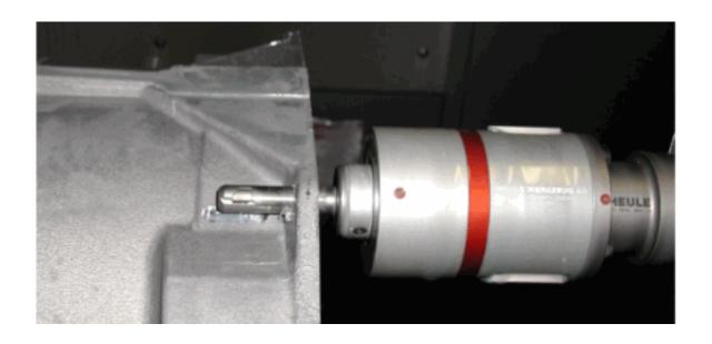
This manufacturer of heavy equipment components is using the SOLO back spotfacing tool to improve reliability and eliminate rejected parts because of missing spotfaces.
