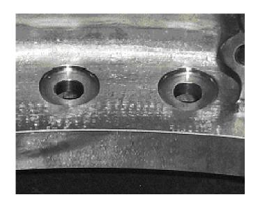
This jet engine services company uses the GH-Z back boring tool to machine these washer seats. The process was to machine the holes in one setup then move and refixture the part for spotfacing. Using the GH-Z to automate the operation on one machine saved moving and fixturing time. A two day process was reduced to hours.
